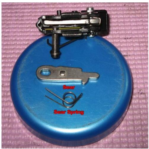
You can now begin removing the sear pin and safety spring. I use a small flat head to push the intermediate lever spring down, releasing tension against the pin. Once you pull the pin out, slowly let the lever spring go. Be careful, there's a good amount of tension on that spring to flip forward and whack your hand. It's also thin and many times can have a sharp end. Use a rag or glove on your hand when doing this to protect your hand from getting whacked by it:
