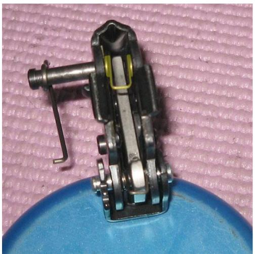
Once the sear spring is in place, position your sear by placing it over the notch and in between the sear spring. Grab that little screwdriver again, press down on the intermediate lever spring to release the tension against the sear pin, and push the pin all the way through:
