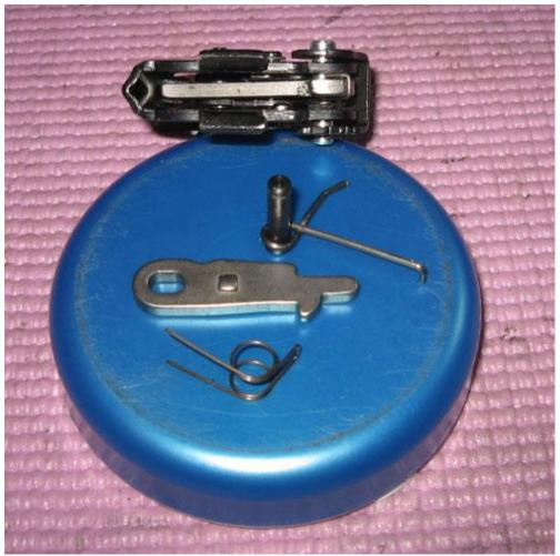
Now we can remove the intermediate lever and its spring. The pin holding those two parts in place also holds the safety lever in place. Remove the highlighted e-clip, then slide it right out. The rest of the parts should now fall out:
