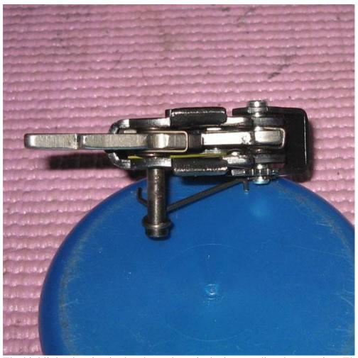
The highlighted spring in the photo above is the intermediate lever spring. That spring is under tension against the sear pin, so you're backing the pin out just enough to remove the sear and sear spring, while still retaining the tension of the intermediate lever spring: Once the sear pin is backed out enough, you can now lift both the sear and sear spring out. Notice the intermediate lever spring is still being held under by the sear pin:
