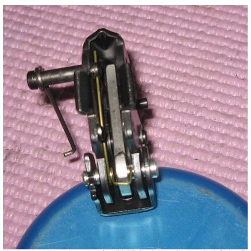
You can now insert the sear spring (highlighted), legs down and tab facing forward:
