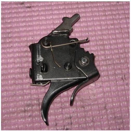
Now that the safety spring is off the safety, we'll remove the sear and sear spring. Start by backing out the pin (yellow) holding the sear and spring inside. Don't take it all the way out, just back it out enough for the sear and spring to clear (you'll see why next:
