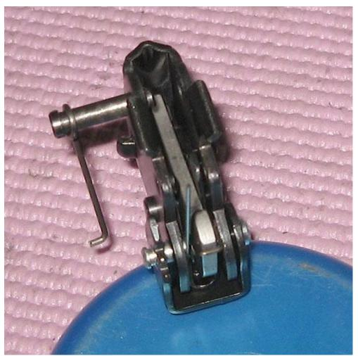
Now take a small flat head screwdriver and carefully work the end of the intermediate lever spring (highlighted) underneath the sear pin as pictured:
